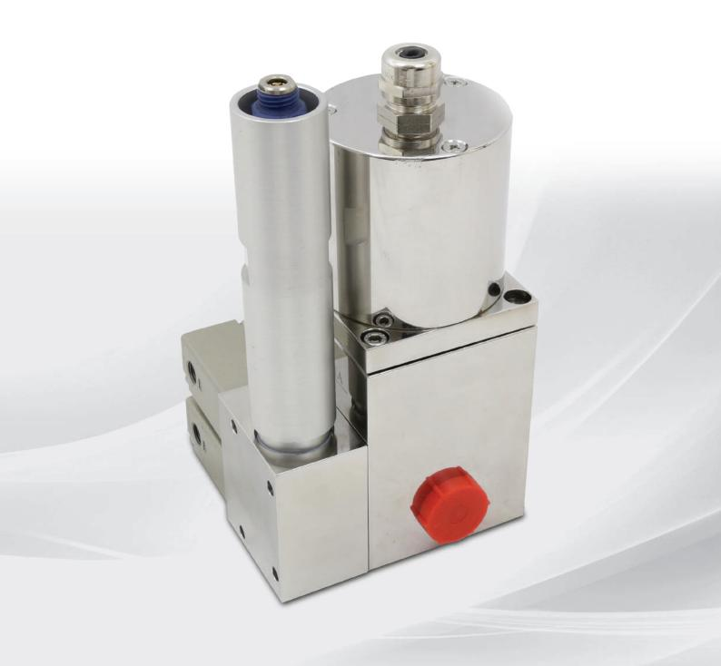
The G29 is a microprocessor controller for the regulation of the viscosity of water based ink. The viscosity measurement is made through a vibration sensor, inline with the ink piping without moving parts. This sensor emits a frequency to the controller that processes the viscosity in seconds (cup ZAHN, FORD etc.) and, then to the water valve, which maintains the value according to the reference signal. The cleaning of the viscometer is made at job end, while washing up.
