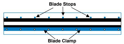
Tighten blade clamp screws from the center to the edges
