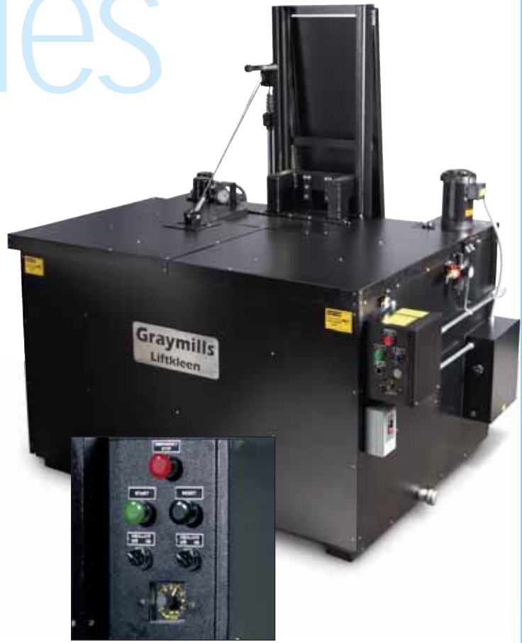
Industrial controls for wash cycle, heater, lift platform agitation and lid.
