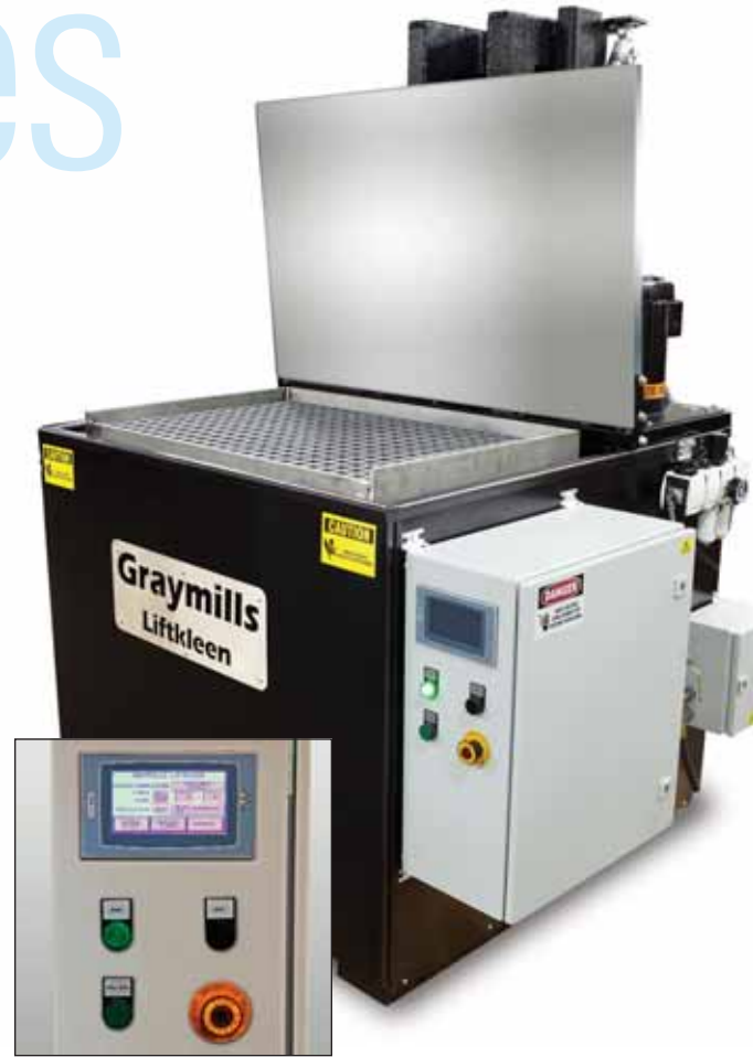
Touch-screen PLC controls for wash cycle, heater, lift platform agitation and lid.
